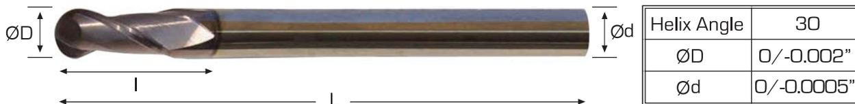
C.N.C. GROUND: 2 or 4 Flutes 10% Co, 0.6 µm grain size
